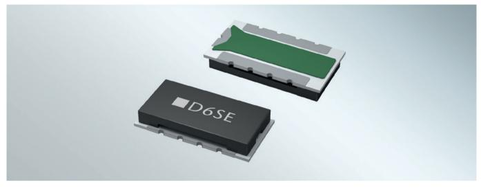
SCHOTT SEFUSE® D6S battery fuses are used in the secondary protection circuit of li-ion batteries to prevent dangerous circumstances of overcurrent and overcharging, and additionally help prevent fires caused by overheating. **D6SE series battery fuses** support rated current of 30A and 45A and are well-suited for high-current applications, such as power tools and E-bikes.
